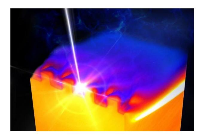
With the aid of the powerful X-ray free-electron laser at SLAC in California, HZDR researchers were able to investigate the plasma processes on the small scales of a few nanometers and femtoseconds on which the turbulent laser interaction with the particles to be accelerated takes place. Credit: Juniks/HZDR
