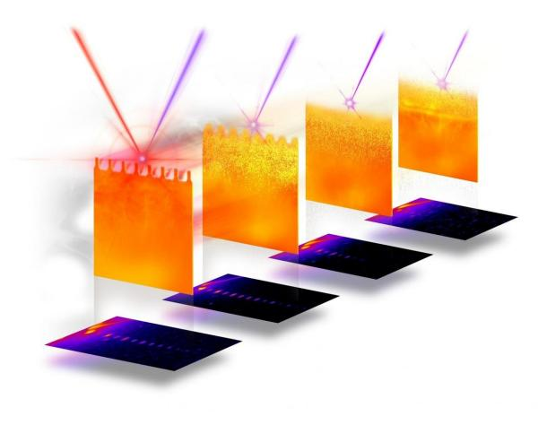
High-intensity laser pulse (red) is focused on a silicon grating target under 45deg; parallel to the grating ridges. The X-ray pulses (blue) probe the laser-plasma dynamics under 90° over time. The scattering patterns below show the complex particle-acceleration processes. Credit: Juniks/HZDR
