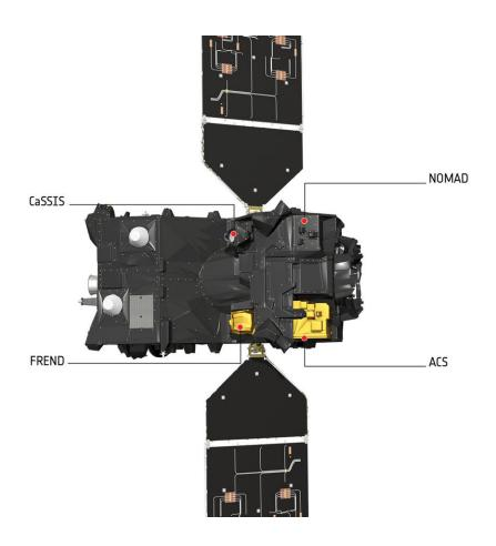
Artist's impression of the ExoMars 2016 Trace Gas Orbiter (TGO) with its instrument packages labelled. Credit: ESA/ATG medialab
