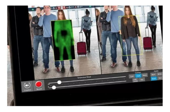
Developed by UK company Thruvision, the body scanners are non-invasive, passively screening individuals for suspicious objects. They work by detecting the absence of the naturally occurring, extremely high-frequency 'terahertz' waves, emitted by anything that is warm – including the human body. The terahertz waves can penetrate clothing and thin plastics or ceramics but not metal or liquid water. However, the Thruvision system can also detect plastics guns and ceramic knives. Credit: Thruvision
