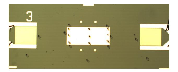
In the device, which is about the size of a fingernail, clusters of diamond nanocrystals (black spots) sit atop a material called a multiferroic. The multiferroic transmits microwave energy into the crystals much more efficiently than other methods. Credit: Dominic Labanowski
