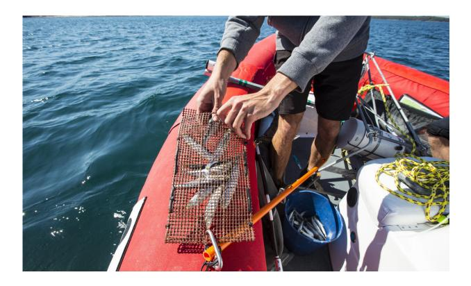
Preparing baited remote underwater video station. Credit: University of Wollongong
