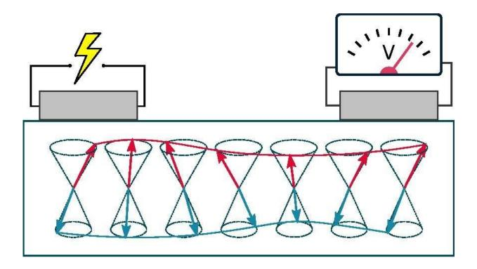
An electrical current in a platinum wire (l.) creates a magnetic wave in the antiferromagnetic iron oxide (red and blue waves) to be measured as a voltage in a second platinum wire (r.). The arrows represent the antiferromagnetic order of the iron oxide. Credit: Andrew Ross
