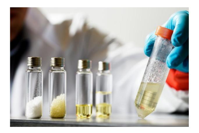
On the foreground two solids and a DES in the making, on the background the DES which has already been formed with a layer of water on top. Credit: Bart van Overbeeke
