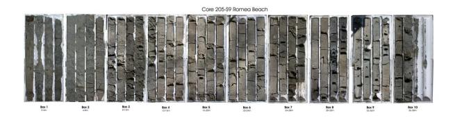
These bars are sections of sediment from one of the cores drilled in the Po Plain in northeastern Italy, about 45 miles south of Venice. Credit: Daniele Scarponi
