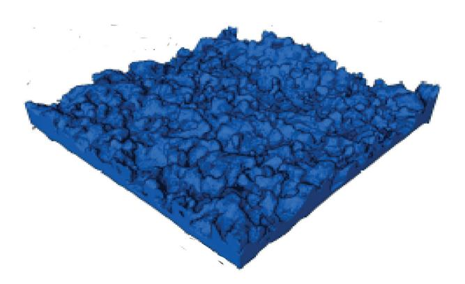
Internal structure of the polyamide thin film. Credit: Enrique Gomez, Penn State
