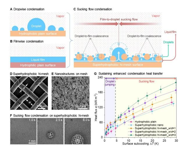
(A) Dropwise condensation on a hydrophobic plain surface. (B) Filmwise condensation on a hydrophilic plain surface. (C) Sucking flow condensation on a hi-mesh surface consisting of the droplet-to-film coalescence and film-to-droplet sucking flow for efficient surface refreshing and droplet growth. (D) Scanning
