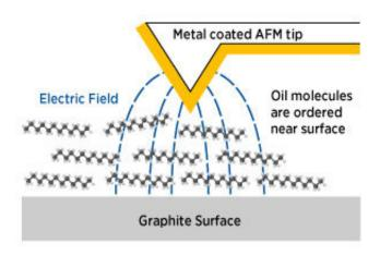
The sharp, metal-coated tip of an AFM can apply very high electric fields across liquid molecules (in this case an oil) right next to a surface. Credit: A\*STAR Institute of Materials Research and Engineering
