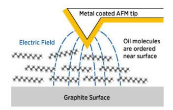
The sharp, metal-coated tip of an AFM can apply very high electric fields across liquid molecules (in this case an oil) right next to a surface. Credit: A\*STAR Institute of Materials Research and Engineering
