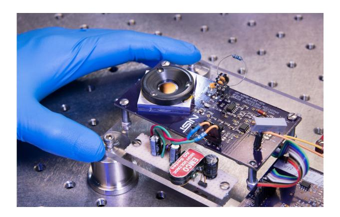
A prototype of the smart mirror. Laser light bounces off the highly reflective surface of a silicon plate, visible in the middle of a thick black ring of plastic. Credit: Jennifer Lauren Lee/NIST
