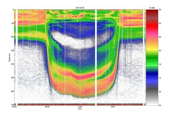
This echogram section displays the acoustic data showing the vertical and temporal distribution of fish within a 24-hour cycle. Contouring represents the presence (orange) and absence (white) of fish within the water column. Fish are retreating to 400 and 600 meters depth during the day and spending time in the upper 200 meters at night. The almost vertical lines show the fish swimming down at sunrise and up at sunset. Credit: KAUST
