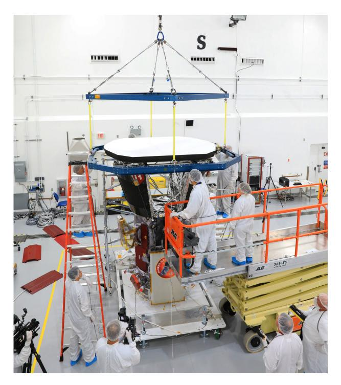
In the Astrotech processing facility in Titusville, Florida, near NASA's Kennedy Space Center, on Wednesday, June 27, 2018, technicians and engineers use a crane to install the heat shield on NASA's Parker Solar Probe. Credit: NASA
