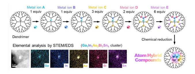
Five metal elements are blended here in a small cluster on a one-nanometer scale. Credit: Takamasa Tsukamoto
