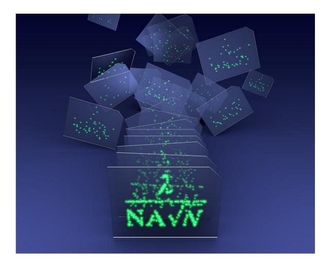
Many different measurements, each containing a few light-emitting points, are combined to form a single image with a high resolution. The formula indicates the uncertainty with which a single molecule can be located. Credit: TU Delft/Bernd Rieger
