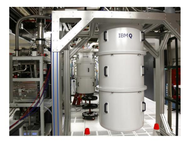
This Feb. 27, 2018, photo shows a quantum computer, encased in a refrigerator that keeps the temperature close to zero kelvin in the quantum computing lab at the IBM Thomas J. Watson Research Center in Yorktown Heights, N.Y. Describing the inner workings of a quantum computer isn't easy, even for top scholars. That's because the machines process information at the scale of elementary particles such as electrons and photons, where different laws of physics apply. (AP Photo/Seth Wenig)
