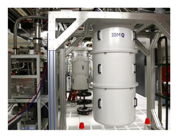
This Feb. 27, 2018, photo shows a quantum computer, encased in a refrigerator that keeps the temperature close to zero kelvin in the quantum computing lab at the IBM Thomas J. Watson Research Center in Yorktown Heights, N.Y. Describing the inner workings of a quantum computer isn't easy, even for top scholars. That's because the machines process information at the scale of elementary particles such as electrons and photons, where different laws of physics apply. (AP Photo/Seth Wenig)
