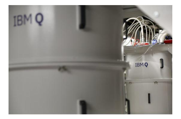
This Feb. 27, 2018, photo shows a quantum computer, encased in a refrigerator that keeps the temperature close to zero kelvin in the quantum computing lab at the IBM Thomas J. Watson Research Center in Yorktown Heights, N.Y. Describing the inner workings of a quantum computer isn't easy, even for top scholars. That's because the machines process information at the scale of elementary particles such as electrons and photons, where different laws of physics apply. (AP Photo/Seth Wenig)
