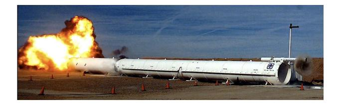
Sandia National Laboratories researchers are using a blast tube to help validate computer modeling and demonstrate the impact of shock waves on nuclear weapons. Credit: Sandia National Laboratories
