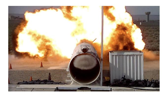
Sandia National Laboratories researchers are using a blast tube to demonstrate how well nuclear weapons could survive the shock wave of a blast from an enemy weapon and to help validate the computer modeling. Credit: Sandia National Laboratories
