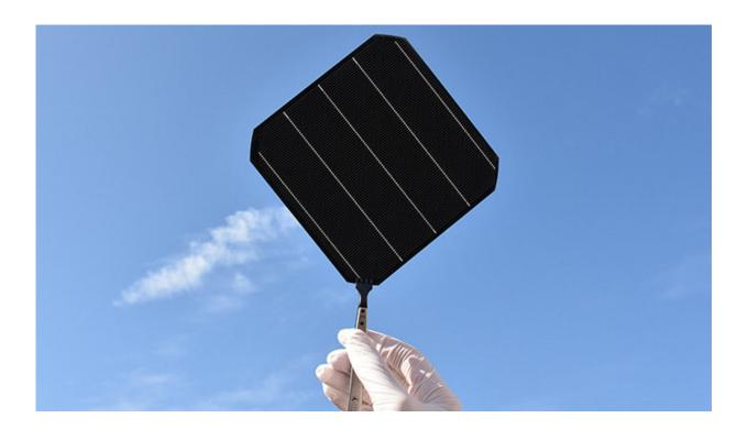
Black PERC solar cell without AR-coating produced at industrial line. Obs. the substrate is multicyrstalline silicon despite the rounded corners. Credit: Hele Savin's research group / Aalto University
