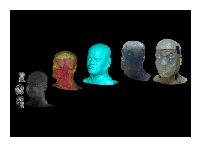
From a 3T MRI dataset and a 3D digital segmented image to a 3D-printed prototype. Credit: RF Research Facility
