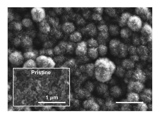
This scanning electron microscope image shows the carbon cathode of a carbon-dioxide-based battery made by MIT researchers, after the battery was discharged. It shows the buildup of carbon compounds on the surface, composed of carbonate material that could be derived from power plant emissions, compared to the original pristine surface (inset). Credit: Massachusetts Institute of Technology
