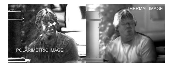
Researchers demonstrate an example of human identification using conventional and polarimetric thermal cameras. The thermal polarimetric image allows for fine facial details to emerge, researchers said. Credit: US Army
