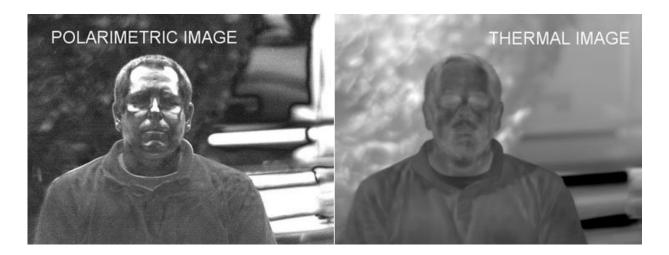
Army researchers show an example of human identification using conventional and polarimetric thermal cameras. The thermal polarimetric image allows for fine facial details to emerge. Credit: US Army
