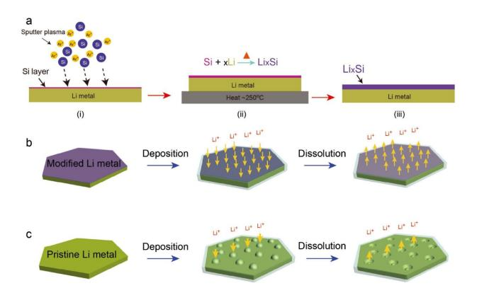
Schematic representation of the preparation process and electrochemical behavior of LixSi-modified lithium foil. Credit: UNIST
