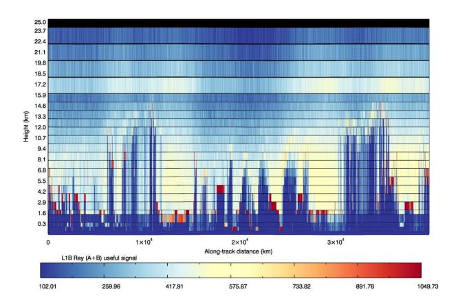
Following the launch of Aeolus on 22 August, this extraordinary satellite is not only emitting pulses of ultraviolet light from its laser, but has also measured light backscattered from air molecules and cloud tops. The measurements show a full orbit around Earth, from the Arctic to the Antarctic, and back. For calibration purposes the signal backscattered from Earth's surface is used, which is also seen in these results. Credit: ESA/ECMWF
