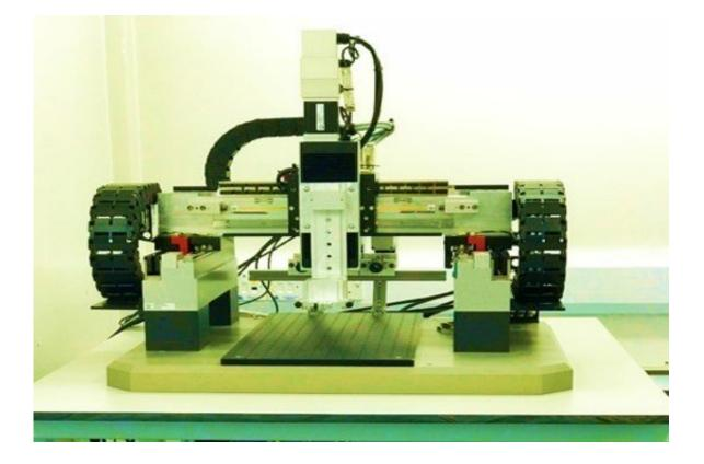
The 3D printing setup – a three axis stage based direct write instrument with one or more syringe pumps to precision dispense inks in a controlled pattern and build 3D structures designed with a customized software. Credit: RoboCAD, 3D Inks, LLC, doi:10.1088/1748-605X/aad2a9
