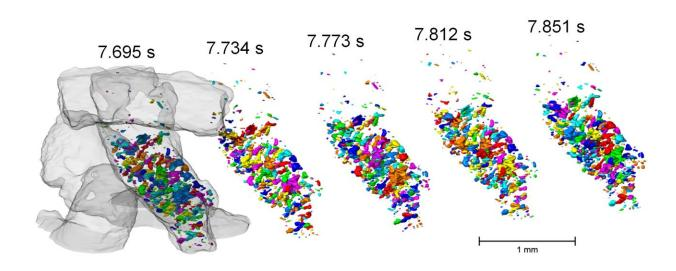
Granules of aluminium (grey) become a metallic foam when heated. The tompgraphies document the evolution of pores with time. Credit: HZB
