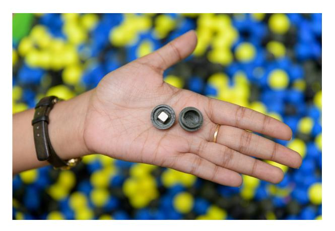
Georgia Tech researchers used 3D printing techniques to create hollow spheres in which loose magnets were placed. The spheres simulated moist soil for testing the work strategies of ants. Credit: Rob Felt, Georgia Tech
