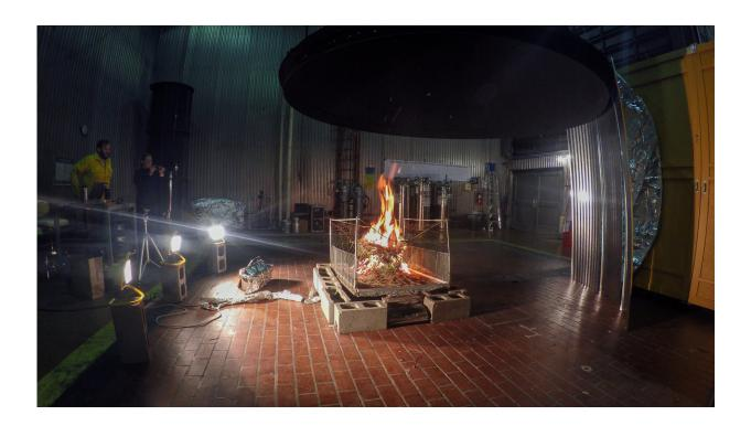
During the Fire Lab study, CIRES and NOAA scientists burned over 100 fires made from various fuels found in the western United States and sampled the emissions continuously with state-of-the art instruments. Credit: Henry Worobec/ University of Montana
