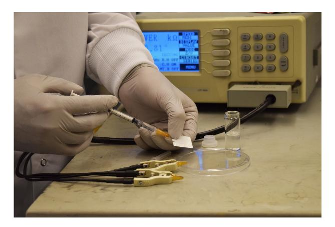
Simply adding a drop of water to a badge engineered by Purdue researchers activates yeast to show radiation exposure as read by an electronic device. Credit: Purdue University image/Kayla Wiles
