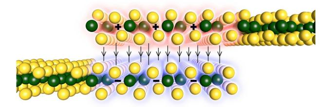
When two monolayers of WTe2 are stacked into a bilayer, a spontaneous electrical polarization appears, one layer becoming positively charged and the other negatively charged. This polarization can be flipped by applying an electric field. Credit: Joshua Kahn
