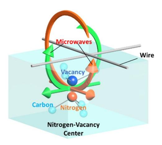
Nitrogen-vacancy (NV) center in diamond with two crossed wires for holonomic quantum gates over the geometric spin qubit with a polarized microwave. Credit: Yokohama National University
