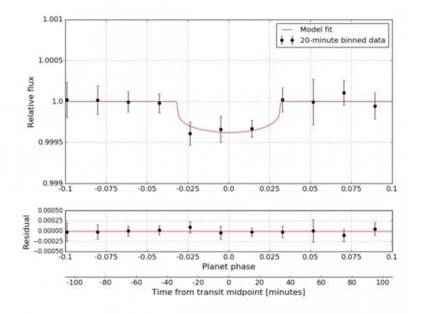
This plot shows the transit lightcurve of 55 Cancri e observed by ASTERIA. Credit: NASA/JPL-Caltech
