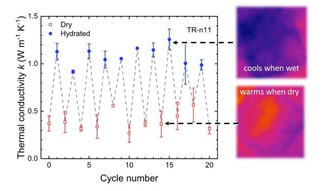
Graph showing cycles of thermal conductivity when material is wet and then dry. Credit: Melik Demirel, Penn State
