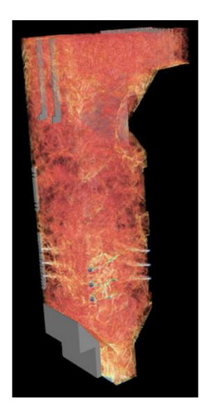
Industrial-scale simulations of novel engineering boiler designs (above) are needed to make them cleaner and more cost effective. Systems such as Frontera will make it possible for the models of such designs to be closer to the engineering systems that are built and to make it possible to use computation to evaluate new designs much more quickly before they are built. Credit: The University of Utah; the University of California, Berkeley; and Brigham Young University
