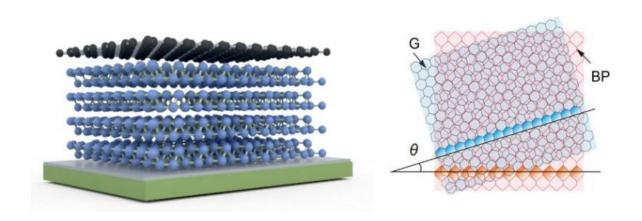
(Left) The lattice mismatch between the monolayer graphene (black) on multilayer black phosphorous (blue) generates PMF on the graphene layer. (Right) The spatial distribution and intensity of the PMF can be tailored by changing the rotation angle between the graphene and black phosphorous. Credit: National University of Singapore
