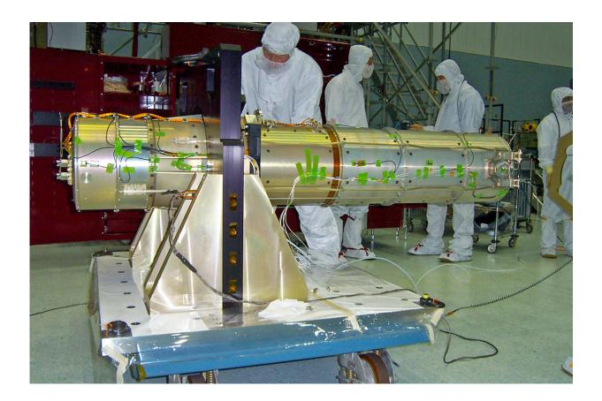
Technicians prepare Swift's UVOT for vibration testing on Aug. 1, 2002, more than two years before launch, in the High Bay Clean Room at NASA's Goddard Space Flight Center in Greenbelt, Md. Credit: <u>NASA's Goddard Space Flight</u> <u>Center</u>
