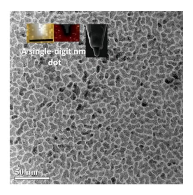
Image of the sub-7-nm nanomagnets. Inset shows bright and dark colors that indicate two distinctive magnetization switching states. Credit: Hong et al. ©2018 American Institute of Physics
