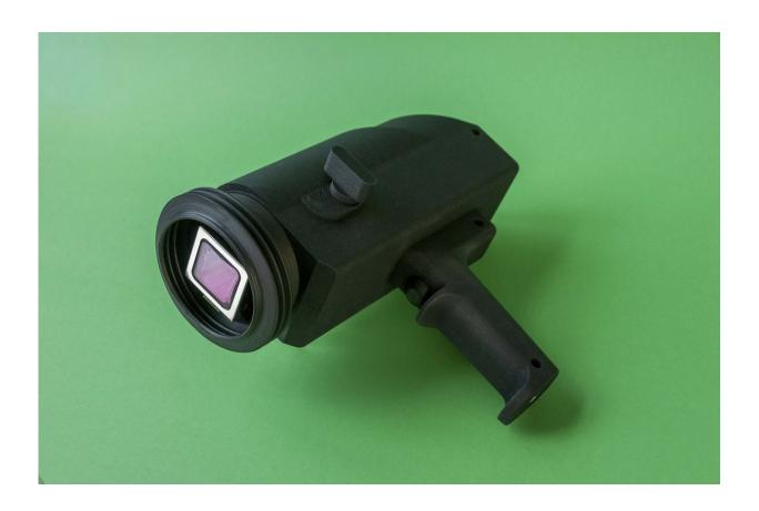
Demonstrator of a mobile measuring gun with luminescent polymeric carrier. Credit: Fraunhofer IST / Falko Oldenburg
