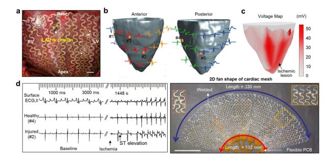
The mesh implanted around a pig's heart was able to record cardiac activity in multiple points. The electrocardiogram (ECG) produced by the device detected an abnormality (ST elevation) caused by an acute heart attack (ischemia). Credit:
