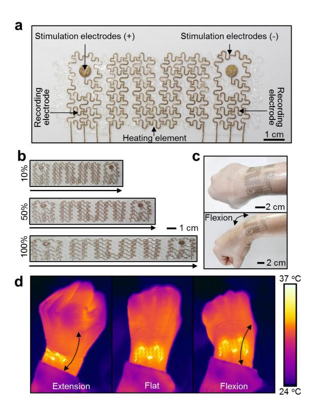
New wearable device capable of recording the electrical activity of the heart and
