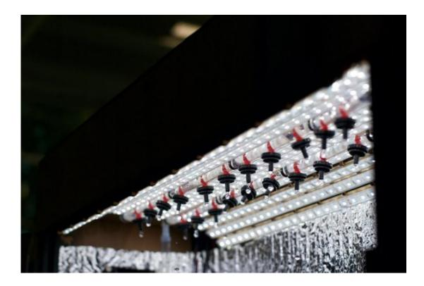
This undated photo provided by Harrison Lin shows the watering and lighting system inside the indoor greenhouse constructed by six engineering students at Rice University. The system measures water for specific vegetables and the lights provide the correct red-blue spectrum needed to grow plants. (Harrison Lin via AP)
