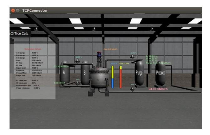
Screen capture shows a chemical processing plant in which critical parameters are rising due to false process data and control commands injected by an attacker. Credit: Georgia Institute of Technology
