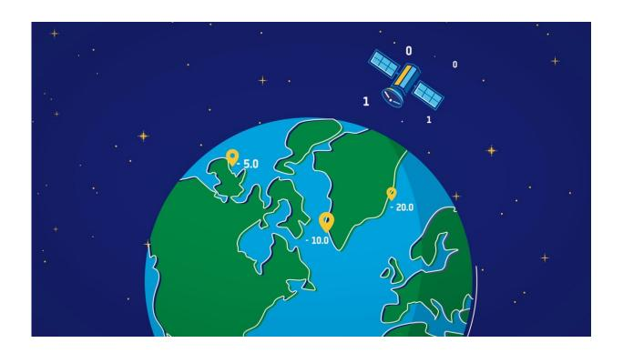
Low-orbiting satellites equipped with light-measuring sensors can record how much light is reflected off the seabed, gathering and updating the information continually as they fly over. Credit: European Space Agency
