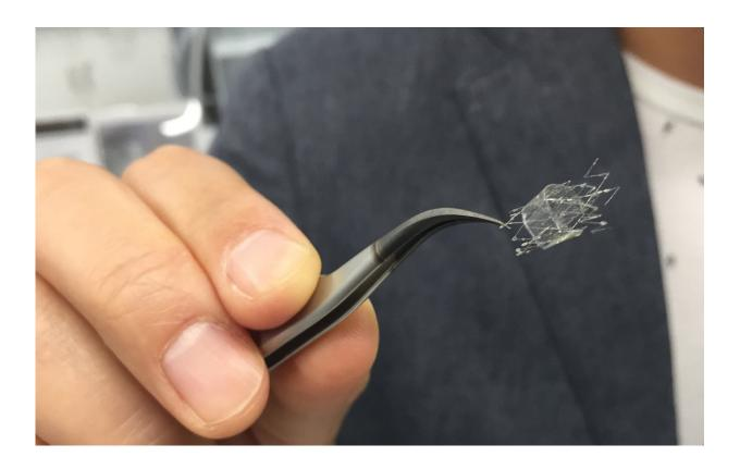
A flow sensor is shown here on a stent backbone. Credit: John Toon, Georgia Tech
