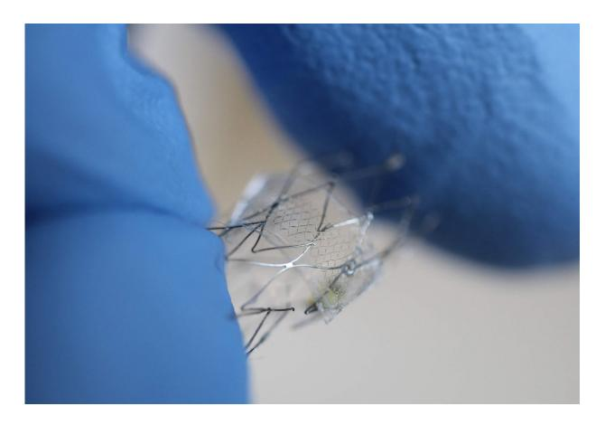
With gloved fingers for scale, a flow sensor is shown here on a stent backbone. Credit: Woon-Hong Yeo, Georgia Tech
