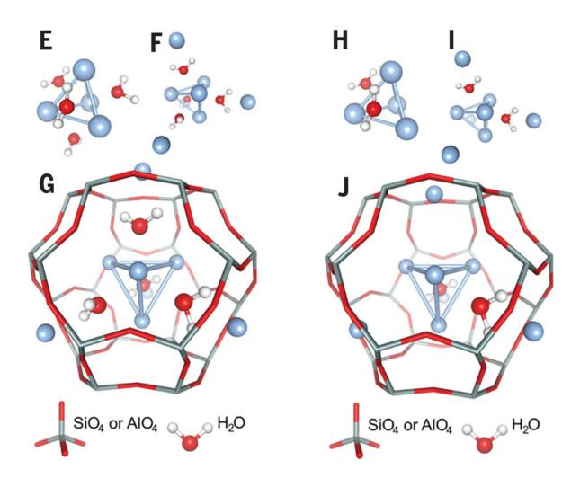
The research provided conclusive evidence that only small clusters of four silver atoms in the form of a tetrahedron and surrounded by water molecules emit light (see blue pyramidal shape in the figure). Credit: © KU Leuven
