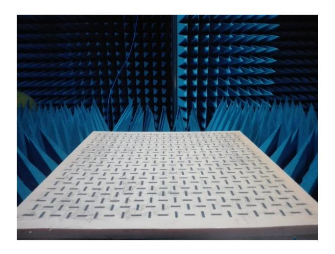
Experimental structure with a strong toroidal dipole response. Credit: ITMO University
