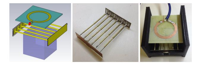
The new MRI coil design. Credit: M. Zubkov et al.
