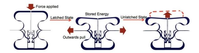
The ratcheting building block that could be embedded in the new materials. After vertical compression, it keeps materials collapsed, and can release their energy on side-ways pull. Credit: Stoyan Smoukov
