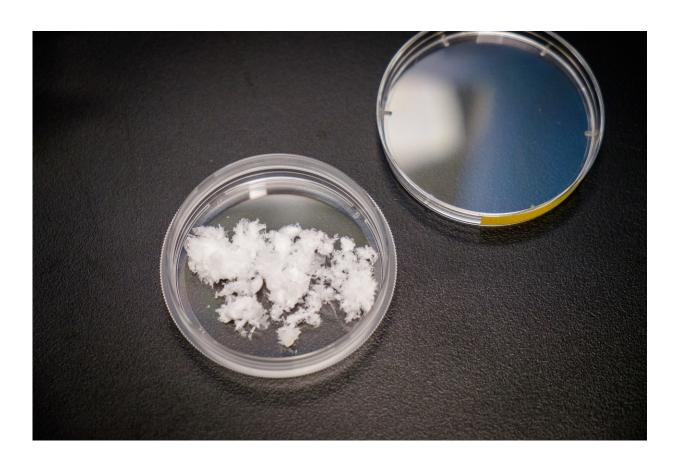
Nanocellulose made from wood pulp used in experiments. Credit: NTU Singapore
