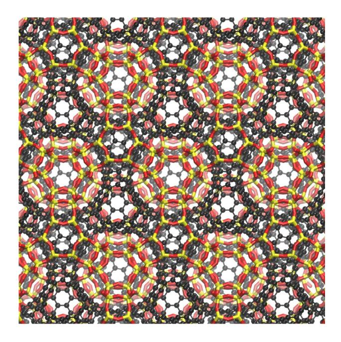
Schwarzite generated by computationally-templating the zeolite FAU. Black spheres are deposited carbon atoms, yellow ribbons are zeolite silicon atoms, and red ribbons are zeolite oxygen atoms. Credit: Yongjin Lee and Efrem Braun (UC Berkeley)
