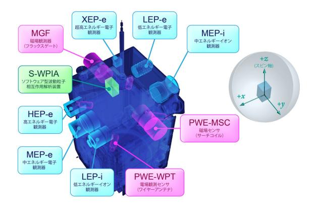
Overview of the Arase satellite and configulation of the sensors implemented on the Arase satellite. Credit: (C)JAXA ERG science team
