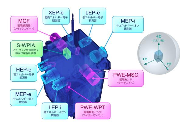
Overview of the Arase satellite and configulation of the sensors implemented on the Arase satellite. Credit: (C)JAXA ERG science team
